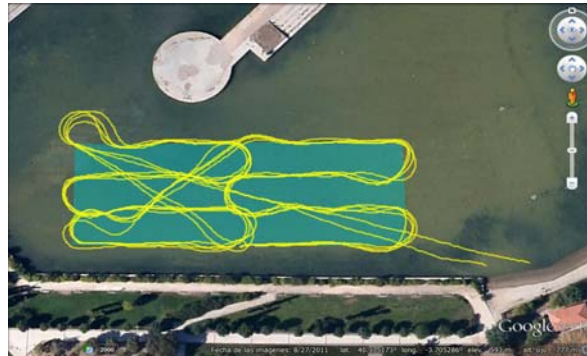
Figure 3: GPS traces of a scan area experiment with the autonomous boats
